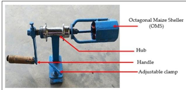
Fig. 3: Modified octagonal Maize Sheller
