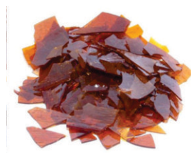
Fig. 10 Hand made shellac
