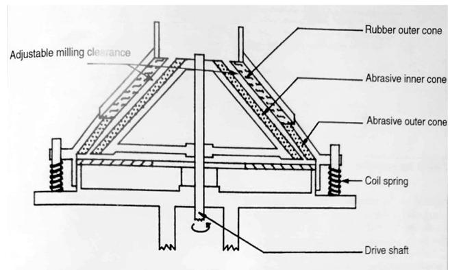
Fig. 3: The milling unit
