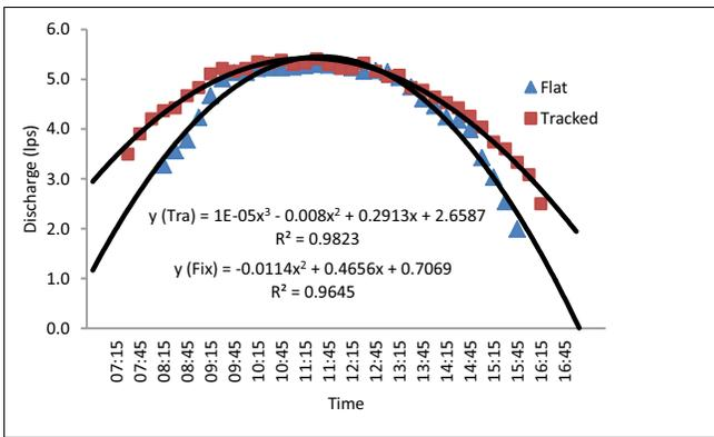
**Fig 3:** Discharges under tracked and fixed array from 3 Hp-3.0kWp solar pumping system over a day during month of April
