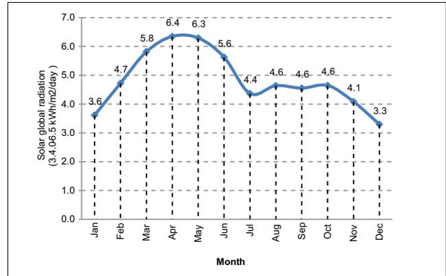
**Fig 1b:** Mean monthly averaged global solar radiation on a cloud free in Eastern region of India
