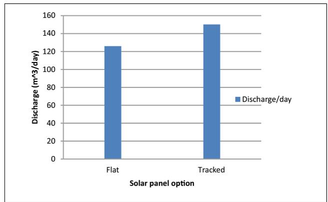
**Fig 4:** The mean monthly averaged daily water output on cloud free day with 3 times manually tracked and fixed array for the month of April
