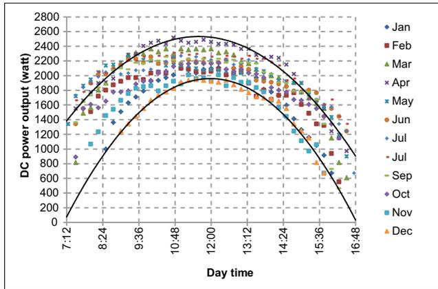
**Fig 2:** Power output from 3.0 kWp operating solar array in Eastern region of India
