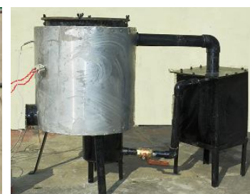
Fig. 2: Vertical cylinder bio-char reactor equipped with external electrical heating system (Gangil and wakudkar, 2013)
