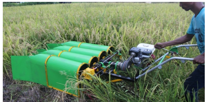
Fig. 9: Photograph of four-row prototype direct ear-head harvester during field testing.
