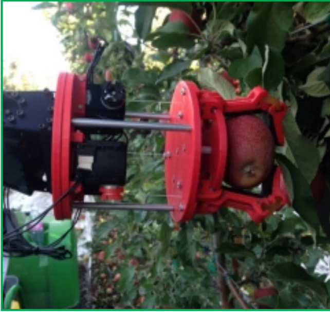
Fig. 2: Apple plucking and twisting with robotic arm (Silwal et al. , 2017)
