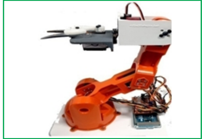
Fig. 4: Robotic arm with cutting type end effector (Masood et al. , 2021)
