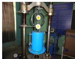
1e: Final measurement for CBR and resilient modulus calculation
