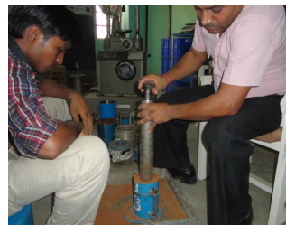
1c: Heavy compaction (5 layers, 55 blows to each layer by 4.89 kg rammer)
