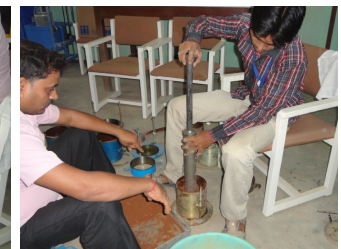
1d: Light compaction (3 equal layers, each being given 55 blows by 2.6 kg rammer)
