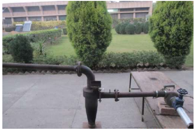
Fig. 5: Experimental set up of Cyclone Gasifier
