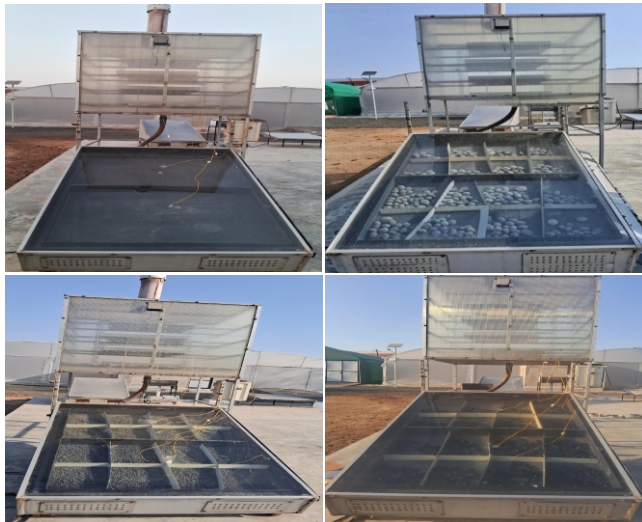
Fig. 3: Different types of TES-based solar drying systems
