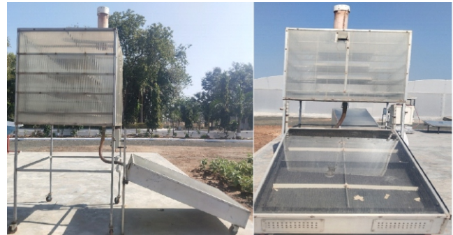
Fig. 1: Indirect passive solar dryer
