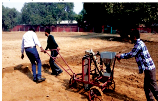
Fig.4 Field evaluation of the gladiolus planter
