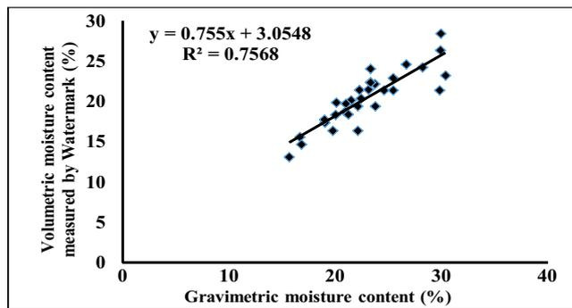
Fig. 8: Regression relationship between moisture measured by gravimetric and Watermark at 15 cm soil depth
