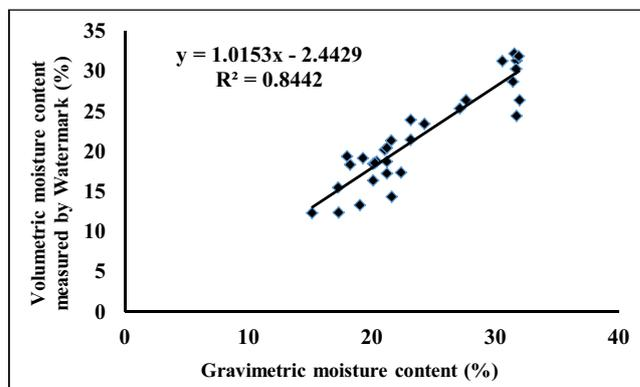
Fig. 11: Regression relationship between moisture measured by gravimetric and Watermark at 60 cm soil depth
