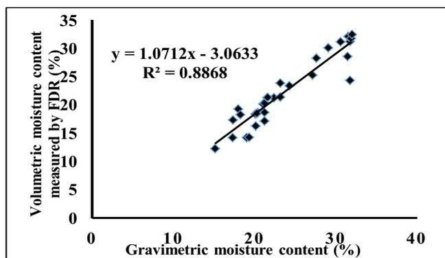
Fig. 6: Regression relationship between moisture measured by gravimetric and FDR sensor at 45 cm soil depth
