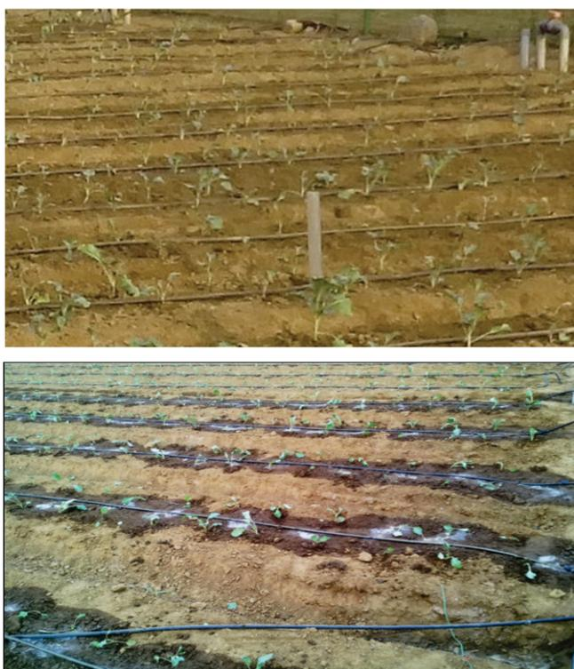
**Fig. 2:** Field installation of a) Access tube for FDR and b) Watermark sensors
