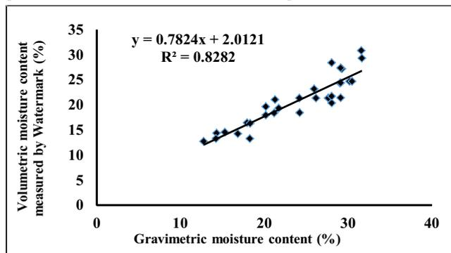
Fig. 9: Regression relationship between moisture measured by gravimetric and Watermark at 30 cm soil depth
