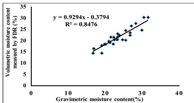
Fig. 4: Regression relationship between moisture measured by gravimetric and FDR sensor at 15 cm soil depth
