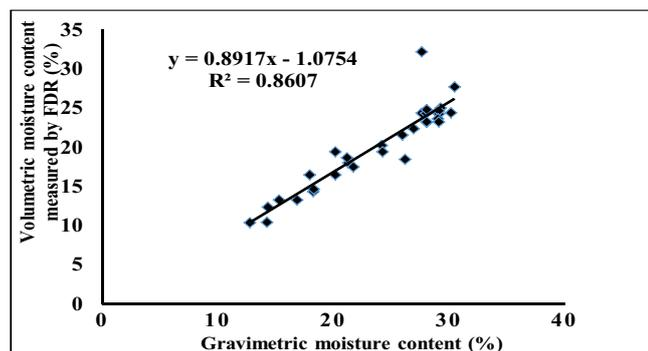
Fig. 5: Regression relationship between moisture measured by gravimetric and FDR sensor at 30 cm soil depth
