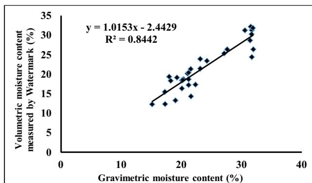
Fig. 10: Regression relationship between moisture measured by gravimetric and Watermark at 45 cm soil depth
