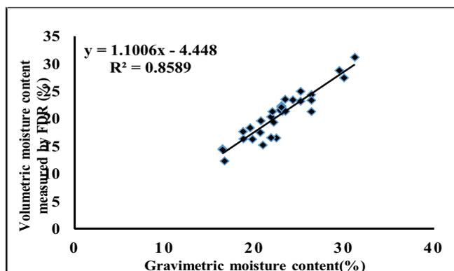
Fig. 7: Regression relationship between moisture measured by gravimetric and FDR sensor at 60 cm soil depth
