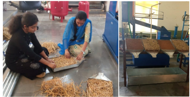
Fig. 2: Rainfall simulator set up for runoff and sediment-analysis
