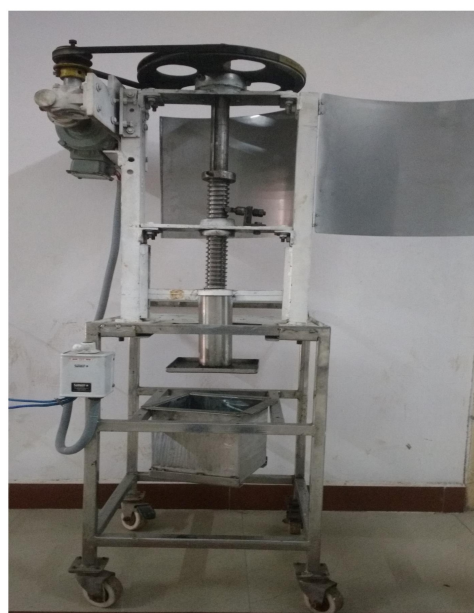
Fig. 4: Prototype murukku extruder
