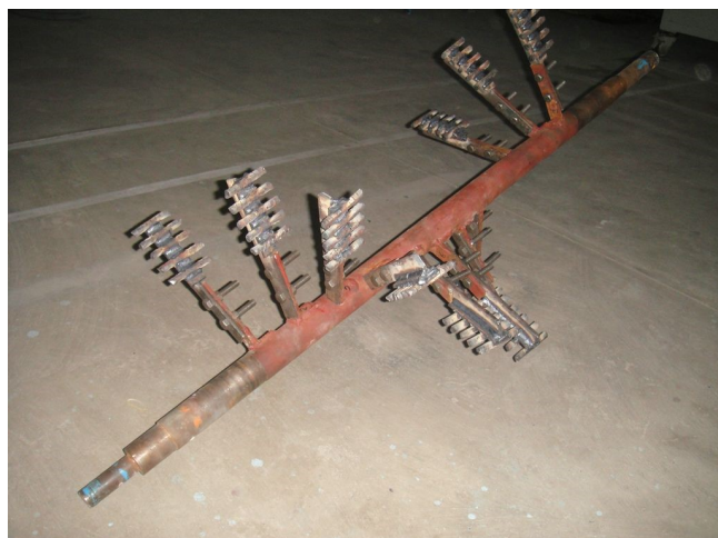
Fig. 3: Modified churning blade mounted on shaft of washing machine
