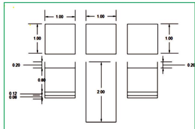
Fig. 2: Plan and elevation of lysimeter setup
